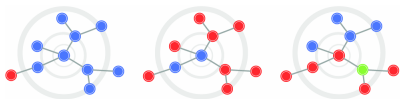
Figure 2. Three chat spaces with the same structure are visualized. Color effectively segments chat spaces by utility. Chat spaces with few unheard messages (left) are not as attention grabbing as a space with mostly unheard messages (middle). When only specific branches have been heard (right), color and layout-based clustering logically segments the space. Concentric rings help distinguish the first message, and function as navigational aid.
